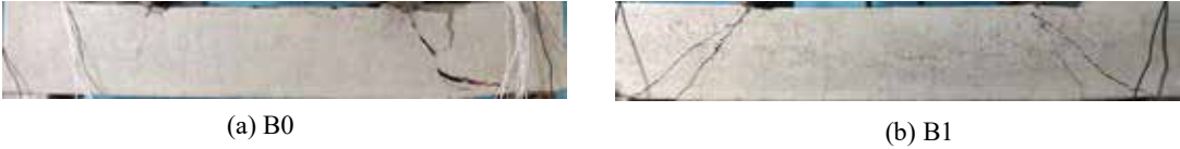
Fig. 2. Photos of crack patterns of tested specimens.
