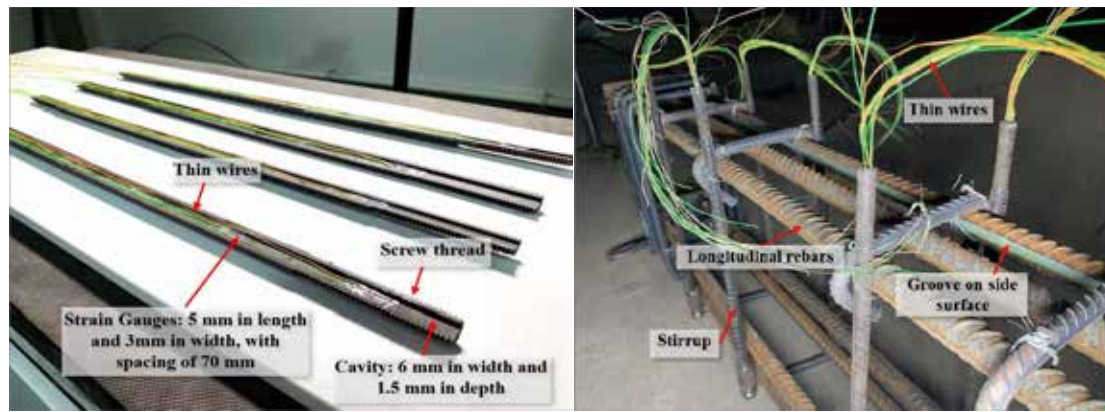
Fig. 1 Cavity inside stirrup legs and steel cage
